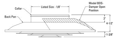
Option: 4800-6 BDS FGBP: Step Down Ceiling Diffuser - w/ R6 Molded Back - 3 Cone - T-Bar - Steel - w/ BDS Damper
